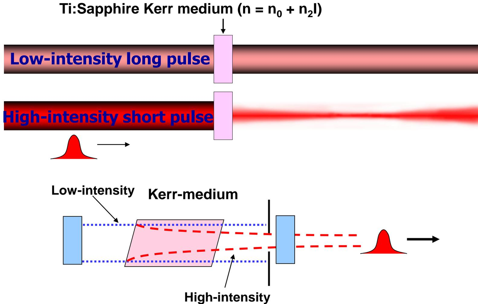
**Higher intensity short pulse is self-focused by the photoinduced lens.**
