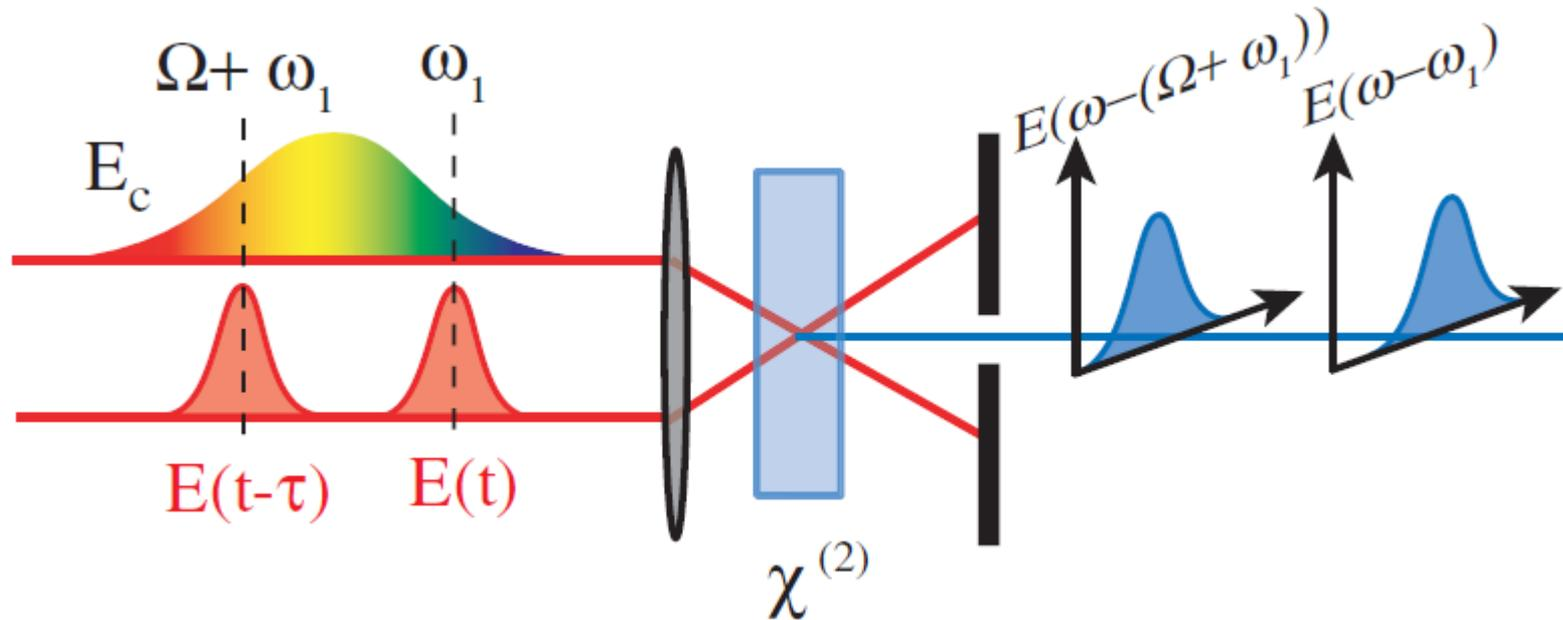
**Spectral interferometry of upconverted pulse at two separated upconversion wavelengths**
