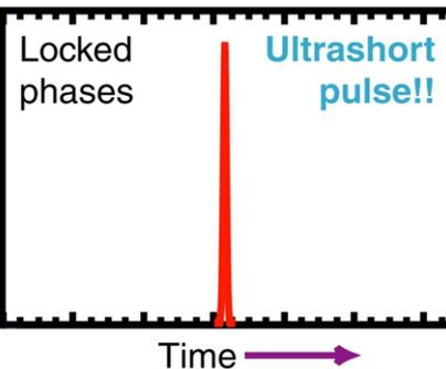
Mode-locking is equivalent to a periodic shutter in the cavity with the round-trip time  $2L/c$  and shutter speed  $2L/\Delta nc$
